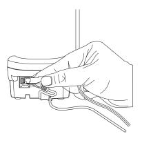
Plug the other end of the cord into the telephone jack on the wall.
